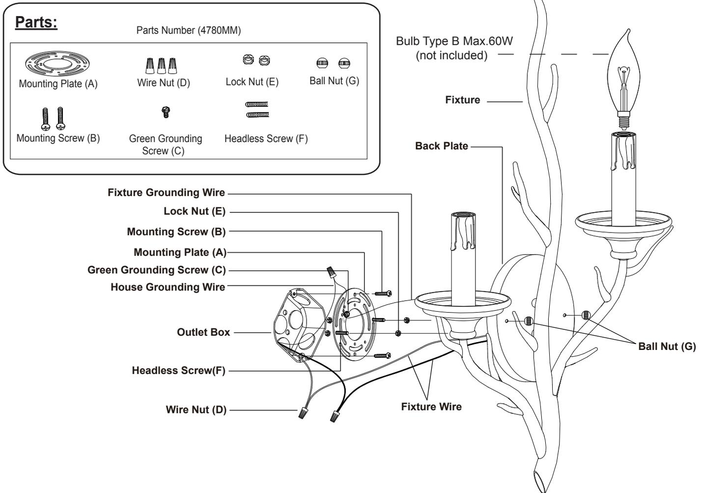
1. Thread two headless screws to the mounting plate, and secure them with four lock nuts (two on each side of the mounting plate). Adjust the length of the headless screws if necessary.
