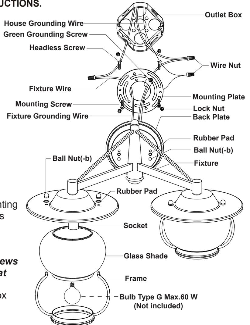
1. Thread two headless screws to the mounting plate, and secure them with four lock nuts (two on each side of the mounting plate). Adjust the length of the headless screws if necessary.
