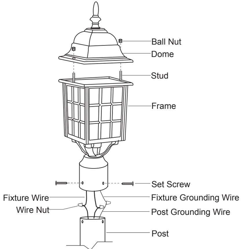
1. Unscrew the ball nuts and remove the dome away from the frame.
