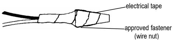
5. Connect the black fixture lead to the black wire in the outlet box.
