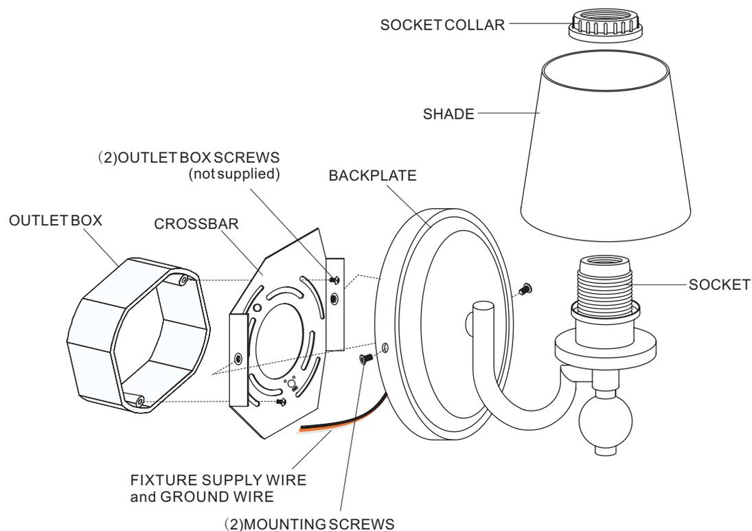
1. Before beginning the installation, carefully unpack and identify all parts, referring to illustration.
