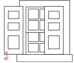
Mounting" above) is required for masonry. Lags provide some adjustment range depending on how far the threads are engaged. Dogs can also be mounted with a round or square post mount. Post mounts have a base with screw holes and a post that extends and engages the hole in the dog. Post mounts are designed for wood surfaces. Finally, some dogs (#88-265 through -268) can be mounted using a sill mount. This attaches to a wood window sill and extends below the bottom of the open shutter.
