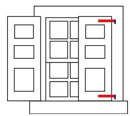
**OFFSET** is the distance between where the hinge mounts and where the pivoting action takes place. Both the hinge and pintle have offset. The offset for the hinge and pintle are usually, but do not have to be, the same. The offset of 13/8 inches for a strap hinge is shown to the right.
