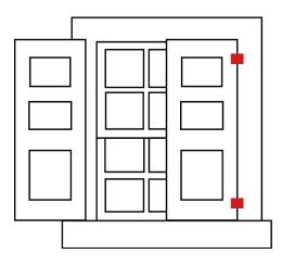
with the hinge in the open position. The pintle half is mounted to the window with the pintle pointing up.
