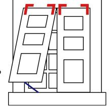
SHUTTER DOGS are traditionally used to hold shutters in the open position. Shutter dogs have a through-hole and are mounted so that they can be rotated to move out of the way of the shutter
