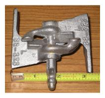
They are commonly used when there is not adequate wood exposed to use an edge-mount hinge. Throw is measured for this hinge in the same way it is measured for a strap hinge. To the left, a throw measurement of  $3\frac{1}{4}$  inches is shown
