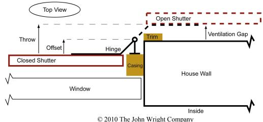
NEW YORK STYLE HINGES are similar in function to strap hinges but work as a right- and left-handed pair, as shown to the right. Offset and throw are determined for these hinges in the same way they are determined for strap hinges. Unlike strap hinges, New York hinges are offered with different offset options. A "new construction" version uses a pintle with 2½ inches of offset and a hinge with nearly zero offset.
