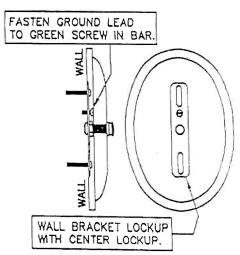
CAUTION — CHAIN HUNG UNITS MOUNTING HOOKS (LOOPS) SHOULD ENGAGE CHAIN ONLY AND NOT ELECTRIC CORD. INSTALLATION SHALL NOT BE MADE ON RADIANT HEATING TYPE CEILING.
