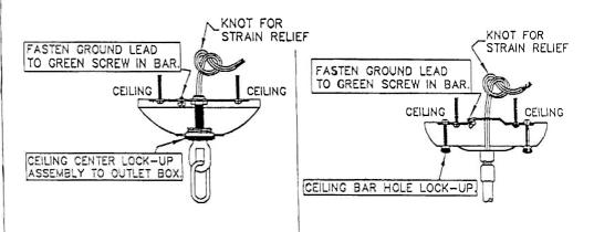
CAUTION — WHEN WIRING CEILING UNITS THE NEUTRAL WIRE (PLAIN) WILL CONNECT TO THE \*WHITE\* LEAD IN CEILING OUTLET. THE TINNED LEAD WILL CONNECT TO THE \*BLACK\* LEAD.
