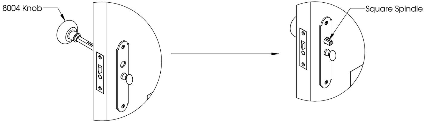
7) Attach lever to interior side of door. Ensure that the spindle rests directly against the interior escutcheon plate (note: the spindle may need to be cut to allow this). Secure the lever to the spindle using the set screw.
