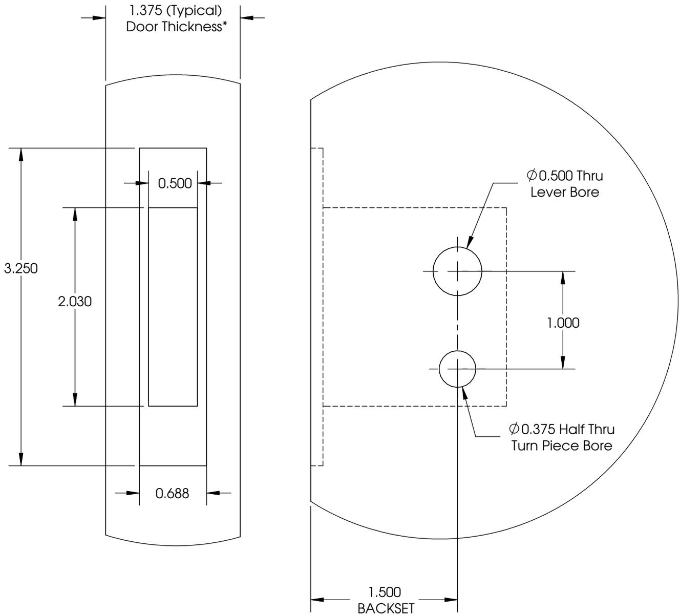
\*While typical door thickness is shown, doors as thin as 1" and as thick as 1 3/4" can utilize the screen door hardware. For doors more than 1 3/8" thick, a thick door kit is required.
