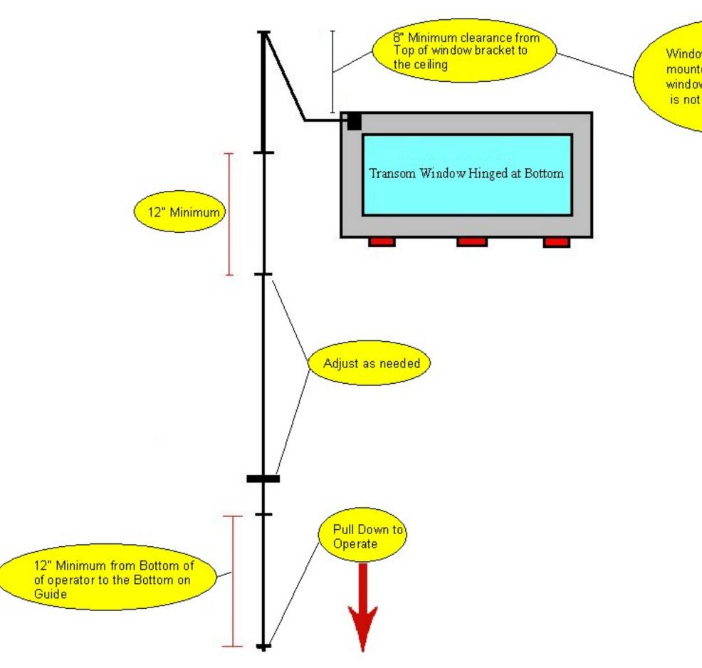
Window Bracket may be mounted lower on the window frame if clearance is not sufficient
