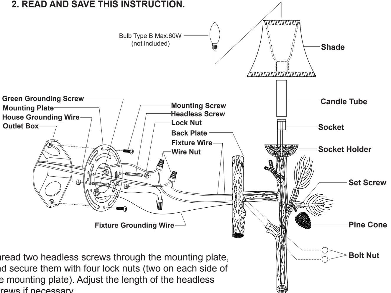
1. Thread two headless screws through the mounting plate, and secure them with four lock nuts (two on each side of the mounting plate). Adjust the length of the headless screws if necessary.
