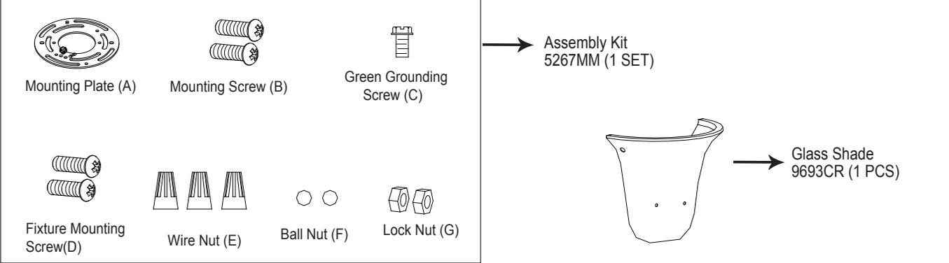
Mounting Plate (A)      Mounting Screw (B)      Green Grounding Screw (C)
