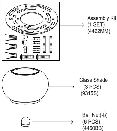
1. Thread two headless screws to the mounting plate, and secure them with four lock nuts (two on each side of the mounting plate). Adjust the length of the headless screws if necessary.
