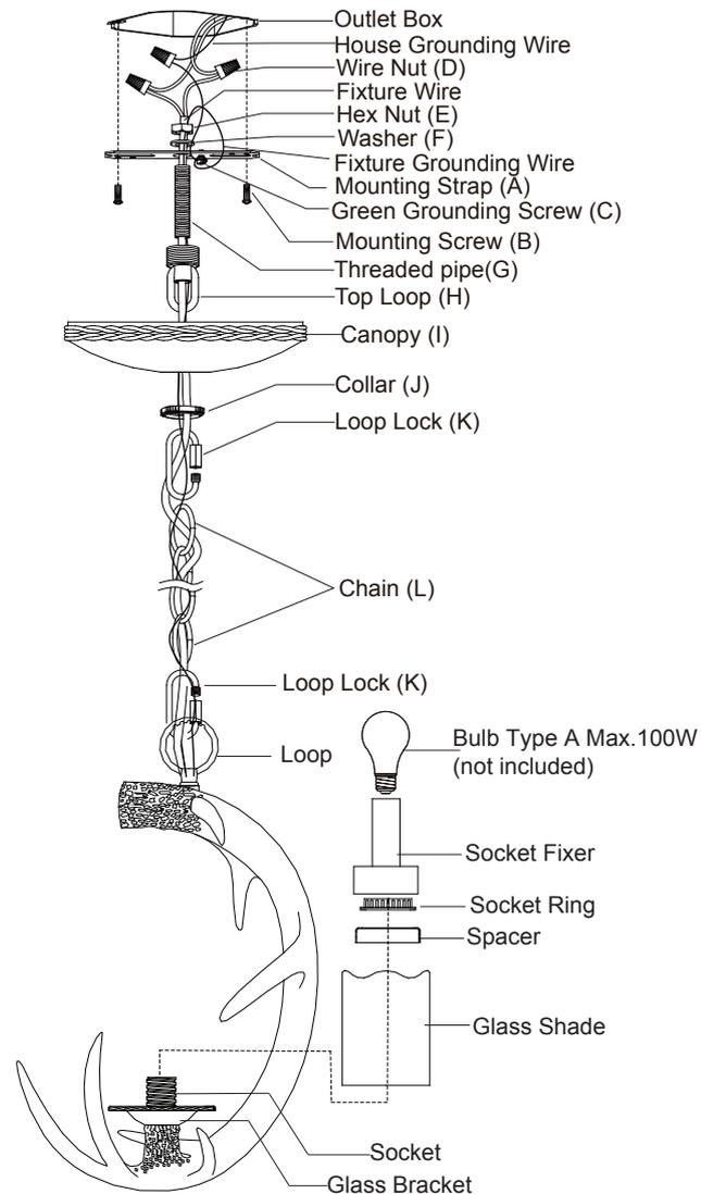
9. Attach the canopy to the mounting strap: insert the top loop through hole, then secure by tightening collar.
