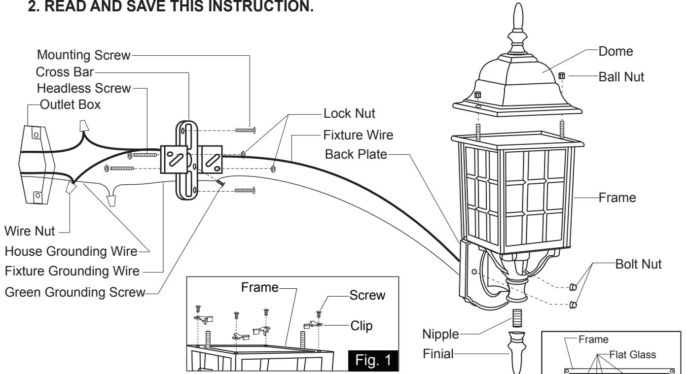
1. Thread two headless screws through the cross bar, then secure them with four lock nuts (two on each side of the cross bar). Adjust the length of the headless screws if necessary.
