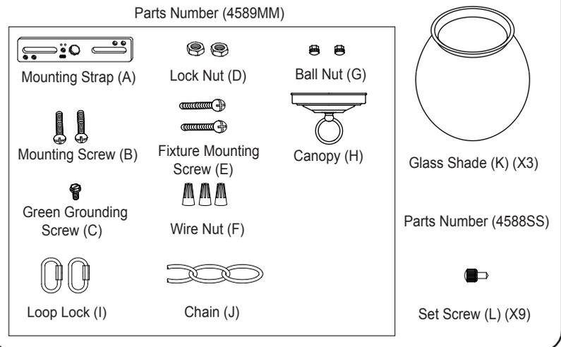
1. Thread two fixture mounting screws to the mounting strap, and secure them with two lock nuts. Adjust the length of the fixture mounting screws if necessary.
