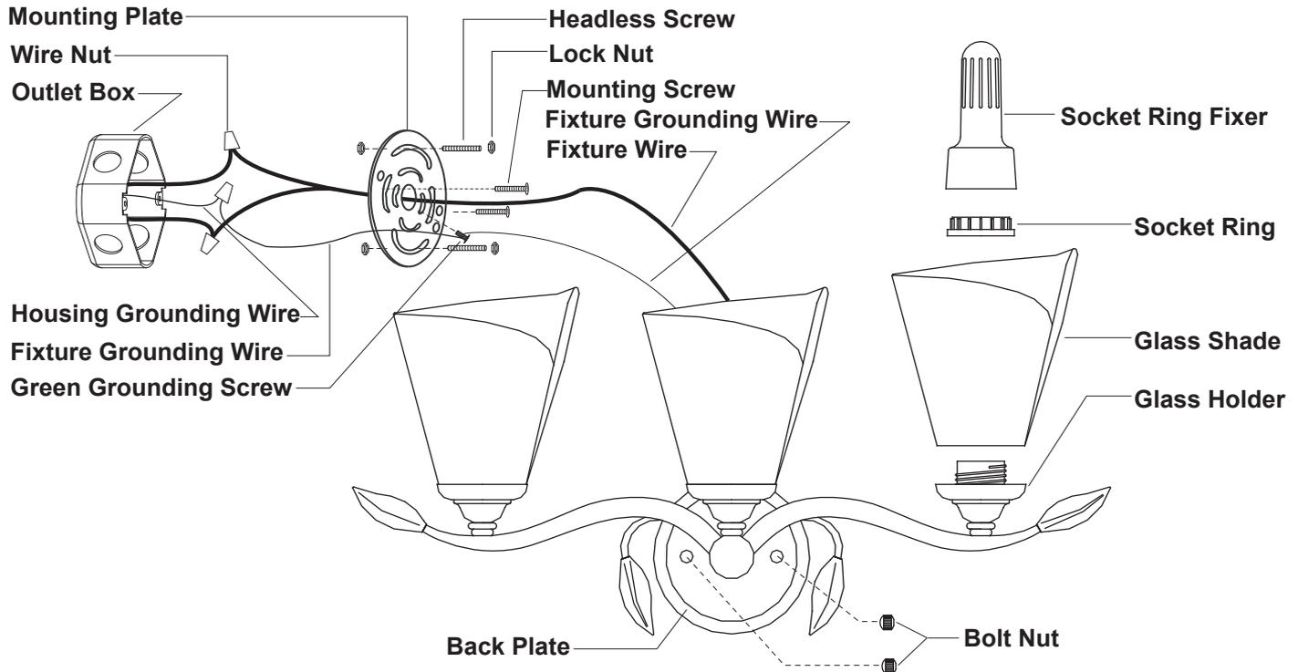
1. Thread two headless screws through the mounting plate, and secure them with four lock nuts (two on each side of the mounting plate). Adjust the length of the headless screws if necessary.
