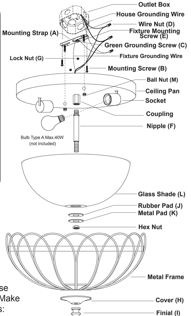
1. Thread two fixture mounting screws through the mounting strap, then secure them with two lock nuts. Adjust the length of the fixture mounting screws if necessary.
