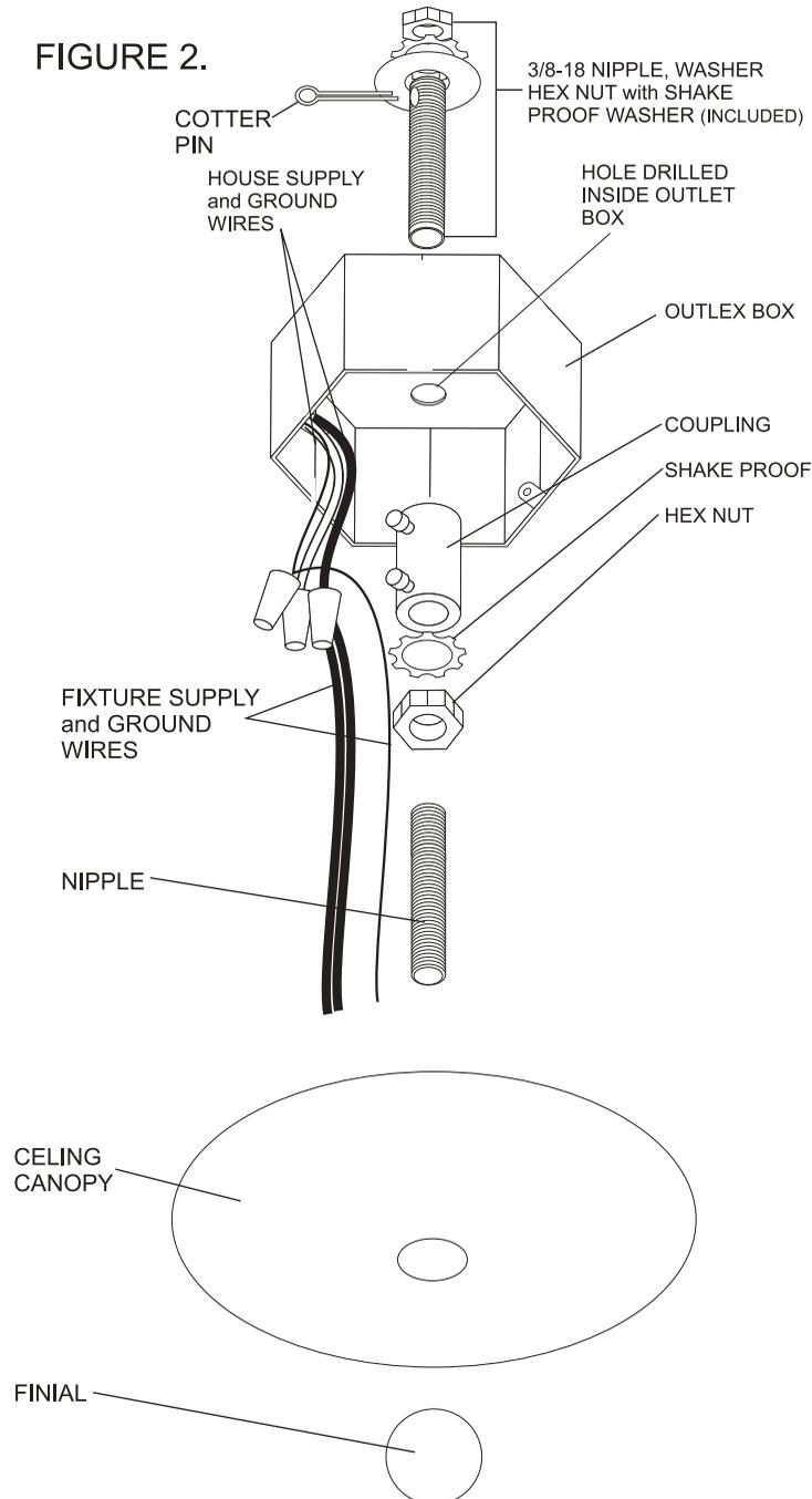
1. Before installing fixture, carefully unpack and identify all parts referring to illustration FIGURE 2. Be sure the power to the installation point is OFF.
