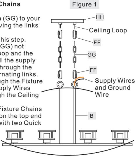
Links (FF) as shown. Lift the fixture and Fixture Chains (GG) up and attach the other ends of the Fixture Chains (GG) onto the Canopy Chain Loop underside of the Ceiling Canopy (HH) with the rest two Quick Links (FF).
