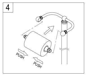
4. Slip the toilet paper into bar and attached the bar to paper holder.
