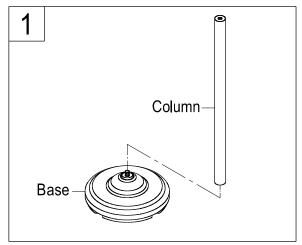
1. Put the base in a level space on ground.
