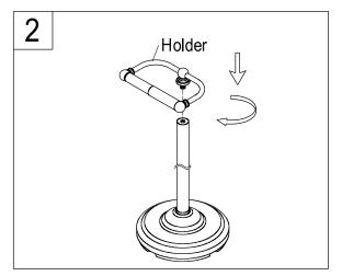
2. Install paper holder into another end of the column tightly with clockwise.
