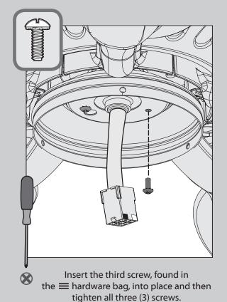
Make sure the upper switch housing is securely attached to the mounting plate. Failure to properly secure all 3 assembly screws could result in the switch housing fixture falling.
