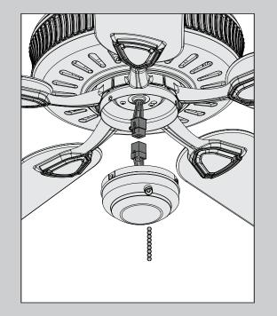
Connect the plugs from the upper and lower switch housings. Make sure to line up the colored markings on the connectors. Lift the lower switch housing up until the holes line up with the screw holes in the upper switch housing. Install the three (3) switch housing screws, found in the  $\equiv$  hardware bag.
