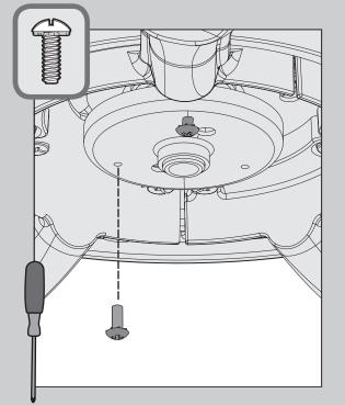
Screw two (2) housing assembly screws from the = hardware bag halfway into the motor housing. It does not matter which two screw holes you choose.
