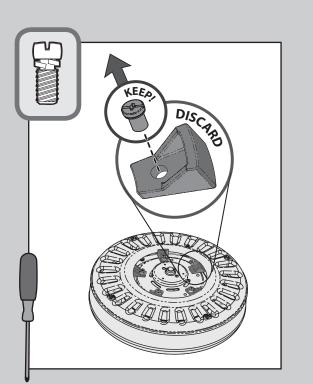
Remove the shipping blocks from the motor. **Save the five screws. They will be needed for blade iron installation.**
