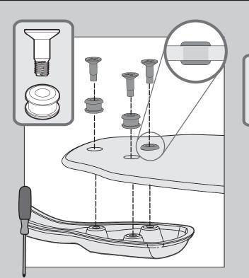
Insert grommets found in the ■ hardware bag into the holes in the blades, then secure each blade to a blade iron with screws found in the ▲ hardware bag.
