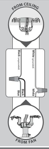
Using orange wire connectors from the  $\bigstar$  hardware bag, connect the black wire (ungrounded) from the ceiling to the black and the blue wires from the fan. Connect the white wire (grounded) from the ceiling to the white wire from the fan.
