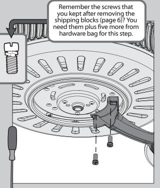
Lightly attach the blade irons to the motor with screws found in the X hardware bag, then securely tighten after both screws are attached.
