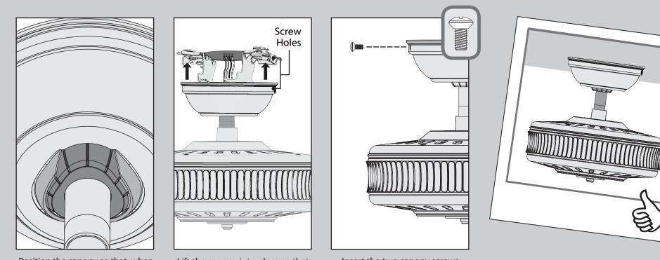
Position the canopy so that, when lifted into place, the canopy fits into the hanging bracket as shown. Lift the canopy into place so that the screw holes are aligned.
