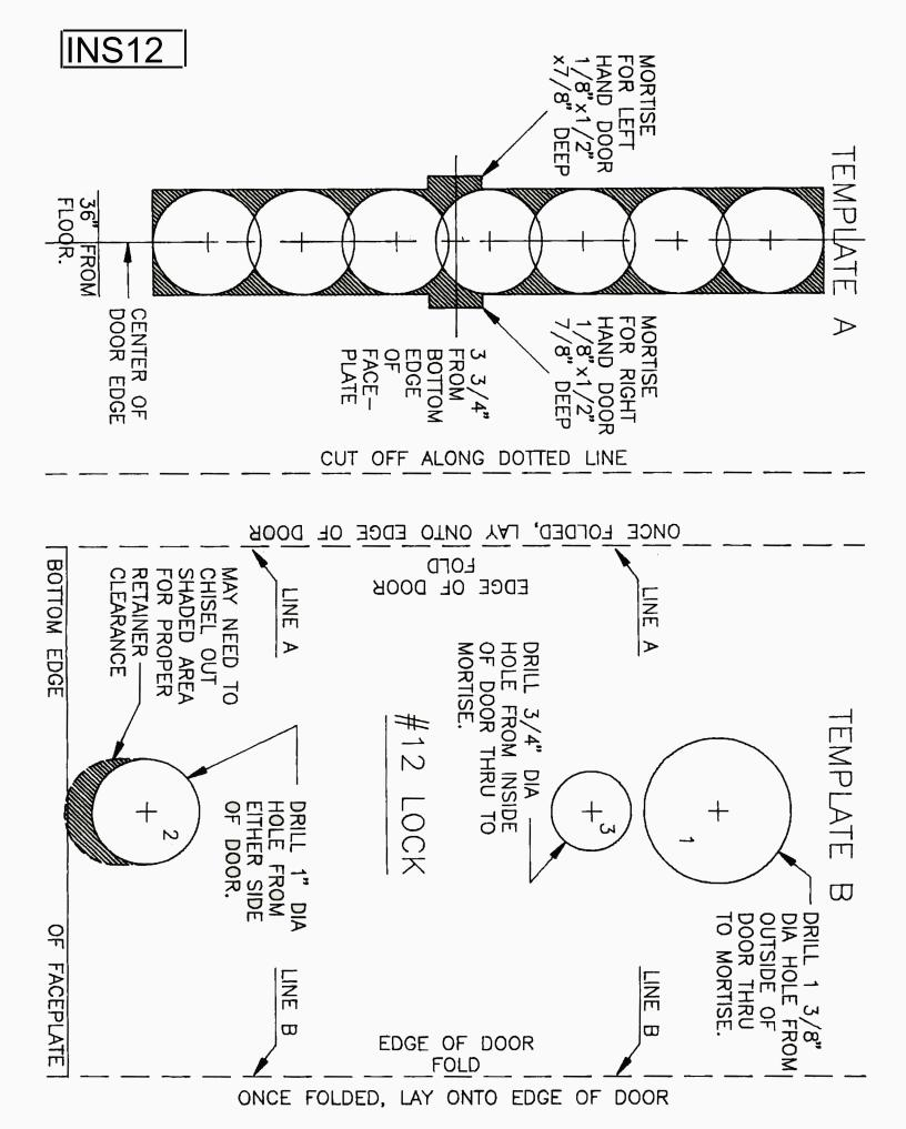
TOOLS REQUIRED: Pencil, tape, awl or nail, drill bits-3/4" and 1-3/8" diameters, drill, Phillips screwdriver, 12" combination square, tape measure, hammer and wood chisels".
